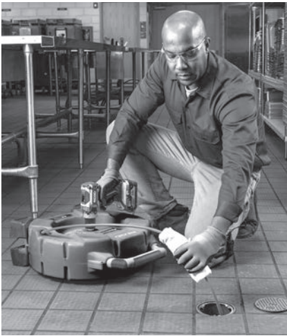
Figure 10 – Applying Lubricant to the Cable Sheath
